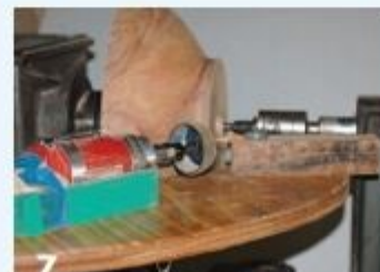
7 Make a table and two sleds, one for an angle grinder and one for a pencil.
