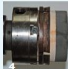
4 Use a rubber pad glued onto a wood block for reverse turning.
