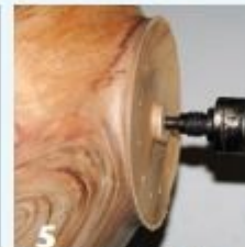
5 The centering pin in the tailstock live center helps center the bowl and hold it onto the lathe.
