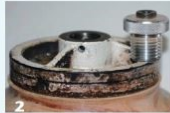
2 The centering tool for reverse turning.
