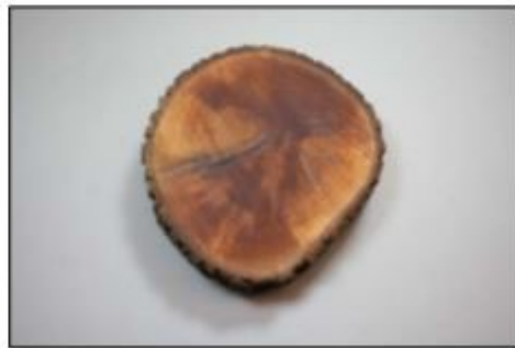
A piece with cracks filled ready to turn
