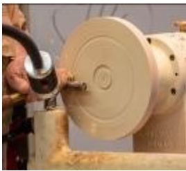
With recess cut, bottom is shaped
