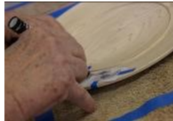
Transfer pen moves pattern to wood
