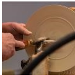
Final scraping of platter
