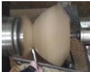
Using spindle gouge for corner
