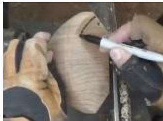
Marking wall thickness
