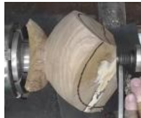
Set to turn interior
