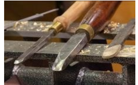
Negative rake scrapers
