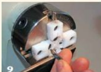
9 With the soft jaws mounted, shape them to best hold your workpiece. Shown here is a recess being cut with a parting tool and threads that will accept the threads of the box being mounted, as shown in the opening image.
