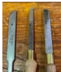
Negative rake scrapers
