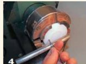
A parting tool is used to form the circular tenon, used later for mounting the jaws to the chuck.
