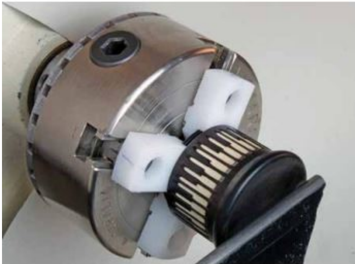
A small turned box is held in threaded soft jaws made of high density polyethylene for finishing the bottom. You can customize your soft jaws according to what the workpiece demands.
