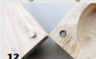
12 The box magnet (right) is recessed \frac{1}{8} ", and the lid magnet (left) protrudes just less than \frac{1}{8} ". The magnetic pull and mechanical fit make this a clever hinge.
