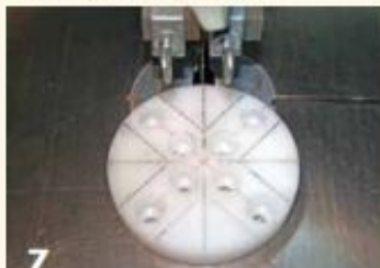
7 Lay out and cut the four jaws on the bandsaw. Before mounting them on the chuck, tighten the backing jaws onto a dowel to eliminate excess play.
