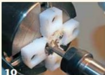
9 With the soft jaws mounted, shape them to best hold your workpiece. Shown here is a recess being cut with a parting tool and threads that will accept the threads of the box being mounted, as shown in the opening image.
