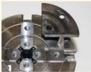
The underside of a typical jaw has a circular tenon that registers in a corresponding groove in the backing jaw. Custom soft jaws are mounted in the same manner.
