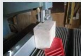
Cutting the lid from the box blank ensures continuous grain flow from lid to body, as well as uniform sizing of parts.
