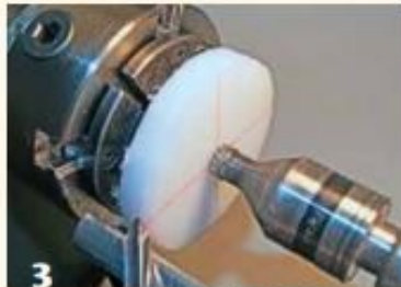
Layout lines are "scratched in" with an awl, then filled with a marker. The HDPE is rough-cut on a bandsaw, then trued on the lathe.
