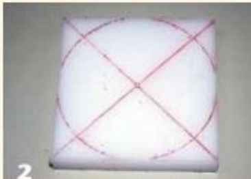
Layout lines are "scratched in" with an awl, then filled with a marker. The HDPE is rough-cut on a bandsaw, then trued on the lathe.
