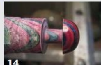
14 After the magnets are installed, the exposed hole on top of the box lid can be concealed with a decorative button of a contrasting wood species.
