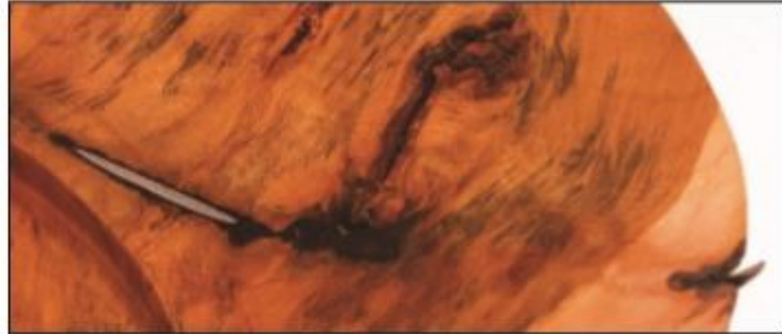
A close-up view of the 10 \frac{1}{2} "-long (27cm) wire embedded in the wood.
