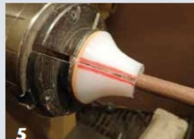
5 In use, be sure this gap (marked in red) is aligned with one of the gaps between the metal jaws of your four-jaw chuck; this allows the collet chuck to close properly.
