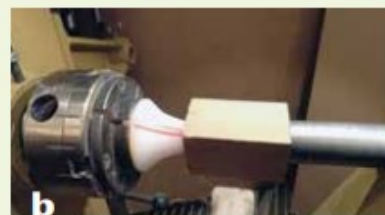
b Mount the dowel/bottle stopper blank in the collet chuck. I used the tailstock ram to ensure the blank was seated properly. Tightening the four-jaw chuck will close the gap in the collet chuck, providing a sufficient hold for smaller projects.
