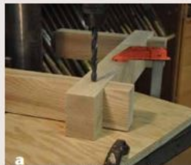
The crossbar-to-post joint is strengthened with carriage bolts, which also help clamp the joint during assembly.
