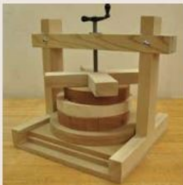
A simple press can hold several turning blanks at once, speeding the process of gluing inlay materials.
