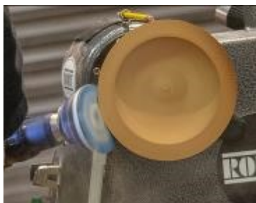
Power sanding the exterior
