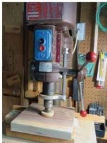
A drill press can apply convenient clamping pressure, here gluing a wasteblock to a turning blank.
