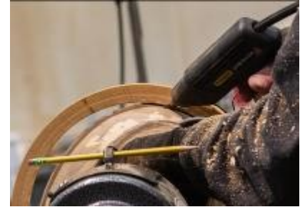
Hot gluing support hoop
