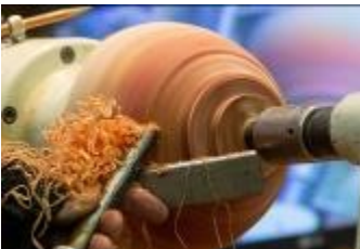
Shaping exterior of NE bowl
