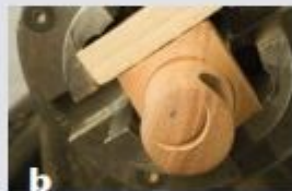
Mount the wood into the 4-jaw chuck with a 1/2" (13 mm) shim to offset the block, creating a new center, noted with a pencil dot.
