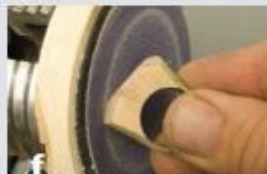
Final sanding is easily done with a shopmade disk sander on the lathe and the grits can be quickly changed.
