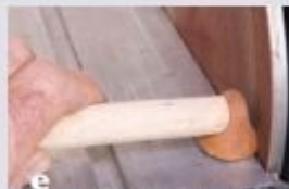
Rectangular forms and facets can be made by holding the ring with a tight-fitting dowel and shaping the top of the ring with a disk sander.
