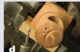
Use a conical rotary-carving tool to create a divot for the dancing man's head.
