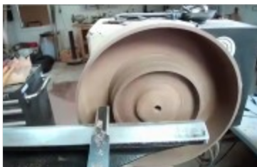
Scraping interior of wall
