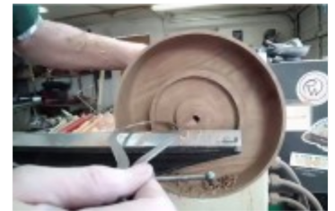
Checking wall thickness
