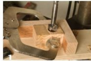
Use a jig for holding the wood when drilling the finger hole.
