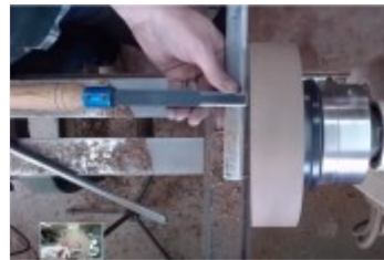
Custom negative rake scraper
