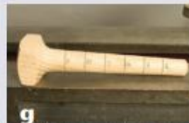
Mark the diameters of your ring-sizing tool with V grooves and burned lines before parting it off the lathe.
