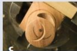
The pencil dot shows the new center. The curved line is the path for the new cut.
