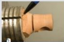
Mark pencil lines on all four sides. These will be used to align the wood for rechunking.
