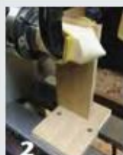
Figure 1: The gauge comprises two main components, shown in red. Part A is fixed, and Part B slides along the bed ways.
