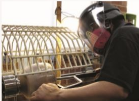
Turning with the wire guard in place, wearing my riot helmet and respirator. The piece, which has multiple cracks, is wrapped in plastic stretch wrap for reinforcement.
