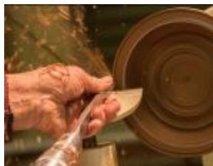
Digging out the trench
