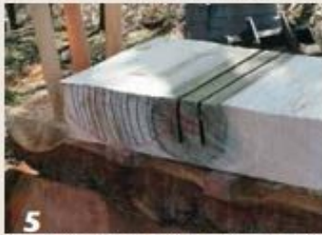
The center section of the log, next to the pith area, yields quartersawn blanks. Depending on the size of the blank and your bandsaw, it may be possible to take the log section straight to the bandsaw for sectioning.
