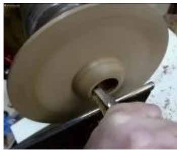
Hollowing with bowl gouge
