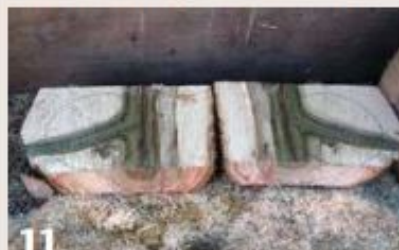
11 Because of the stability of quartersawn timber, the two spindle blanks opposite the limbs are worth coating with wax and setting aside to dry.
