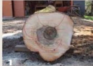
1 The three outlined blanks will all yield stable forms, and the top and bottom blanks should have pleasing grain patterns.
