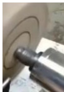
Tenon & base marked out
