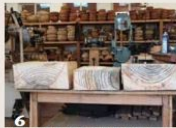
With carefully planned and executed chainsaw cuts, the blanks are ready for the bandsaw table, where the bowl blanks are cut round from the square chainsawed blanks. From left: a flat-sawn, natural-edge-oriented blank (but in this case, with the bark eliminated), a quarter-sawn blank, and a flat-sawn blank.
