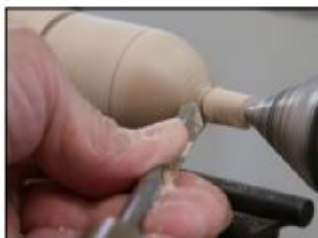
Photo 12 - End the cut with the flute in the 3 o'clock position (closed flute).
