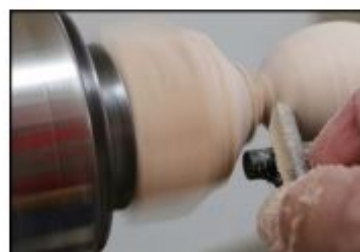
Photo 16 - Finishing the cut on the pointy end.
