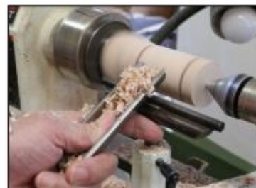
Photo 6 - Roughing to round and final diameter with a spindle roughing gouge.
