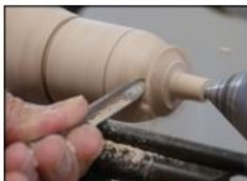
Photo 11 - Rotate the flute as you cut the curve, like cutting a large bead.
