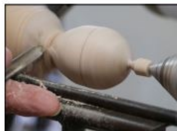
Photo 15 - Make a relief cut - cutting away wood on the headstock side of the blank so that you can get the spindle gouge around the end of the egg.
