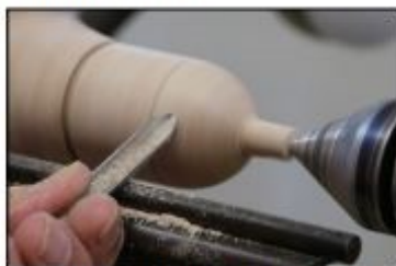
Photo 10 - Start the cut with the bevel on the wood and the flute in the 1 o'clock position (open flute).
