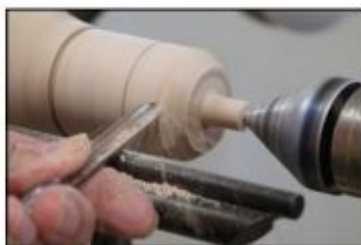
Photo 9 - Cutting from the diameter line to the blunt end of the egg.
