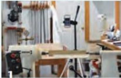
The author's smartphone mounted at ear height near the lathe. There are several apps designed to give instant readings of noise levels.
