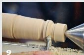
9 The bead is formed by rolling the spindle gouge through an arc, with its flute rotating from 12-to-3 o'clock for the right side of the bead, and 12-to-9 o'clock for the left side.
