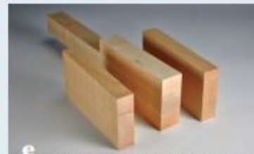
After the five mallet components are milled, the two smaller side pieces of the head are glued to the core first, followed by the larger pieces. If the two small pieces are not perfectly flush with the handle, allow the glue to cure and pass the assembly through a thickness planer before gluing the wider strips in place.
