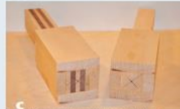
Laminating a blank can produce a mallet with vertical grain around its entire perimeter and yields the most durable tool.
