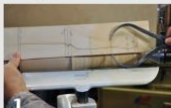
1 A template defines the key features of the mallet, and makes transferring measurements with calipers quick and easy.
