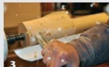
2 Roughing proceeds by cutting from one end of the blank and working in increments back towards the center. Keep an eye on the profile of the rotating blank to see that material is being removed uniformly, and stop the lathe periodically to gauge progress.
