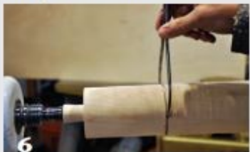
6 The parting tool defines the location and diameter of the bottom of the head.
