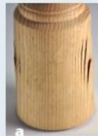
This mallet, made from a single piece of flat-sawn wood, has failed in the sidegrain areas. Note that the visible quarter-sawn area, with wood grain facing out, remains intact.
