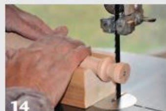
14 Removing a spigot with the bandsaw. Unsupported round stock can catch violently on a bandsaw, ruining the blade and potentially pulling your hand into the teeth—do not attempt this cut without a v-block holding jig.
