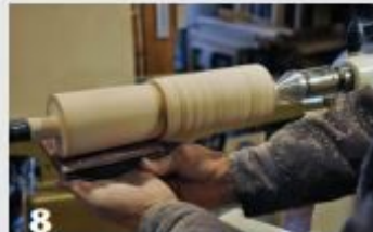
7 The head is shaped with the roughing gouge and sanded flat and true with the aid of a sanding block. Always remove the toolrest for sanding.
