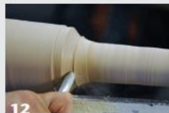
12 Coves connect the bead elements at either end and determine the handle's feel in the hand.
