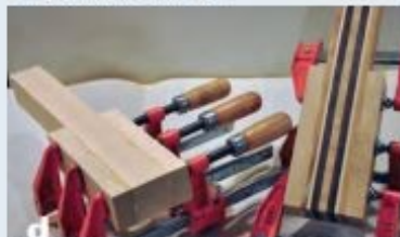
After the five mallet components are milled, the two smaller side pieces of the head are glued to the core first, followed by the larger pieces. If the two small pieces are not perfectly flush with the handle, allow the glue to cure and pass the assembly through a thickness planer before gluing the wider strips in place.
