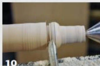
9 The bead is formed by rolling the spindle gouge through an arc, with its flute rotating from 12-to-3 o'clock for the right side of the bead, and 12-to-9 o'clock for the left side.
