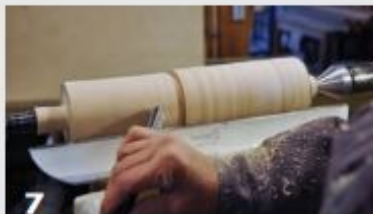
7 The head is shaped with the roughing gouge and sanded flat and true with the aid of a sanding block. Always remove the toolrest for sanding.
