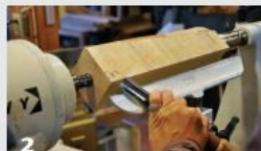
2 Roughing proceeds by cutting from one end of the blank and working in increments back towards the center. Keep an eye on the profile of the rotating blank to see that material is being removed uniformly, and stop the lathe periodically to gauge progress.
