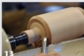
13 Cut the endgrain across the top of the mallet to produce a slightly concave and stable rim on which the mallet will stand. This can be done while reducing the spigot in preparation for parting off.
