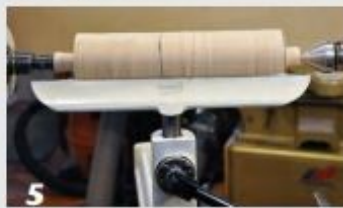
Use a parting tool to define the ends of the mallet and reduce the spigots to about 1" diameter.
