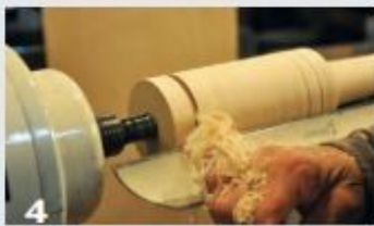
Use a parting tool to define the ends of the mallet and reduce the spigots to about 1" diameter.
