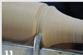
11 The transition from the head to the handle is a combination of decorative elements turned with the spindle gouge.
