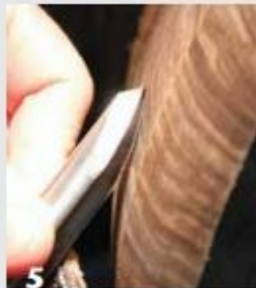
Note the steep angle of the cutting edge to the wood. Close the flute of the gouge, but be careful to apply only one wing, not both.
