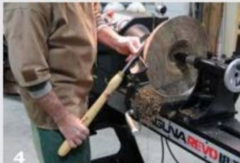
Imagine putting the tool handle in your pocket to achieve the steep angle needed for a shear-scrape.
