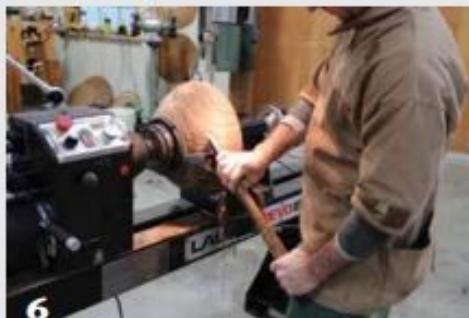
Similar to the gouge presentation, lower the handle of a scraper when used in shear-scraping mode.
