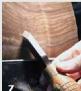
Turn the scraper up on edge (so it is not flat on the toolrest) to achieve the steep cutting angle needed for a clean shear-scrape.
