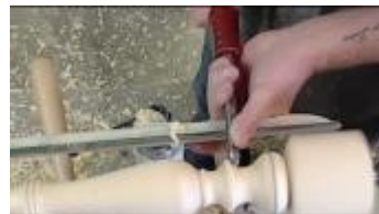
Taking finishing cuts
