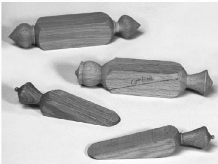
Author's production doorstops (these are of oak to match oak flooring) begin as simple spindle turnings with most of the length left square. Bandsawing them apart diagonally yields two stops from each blank.
