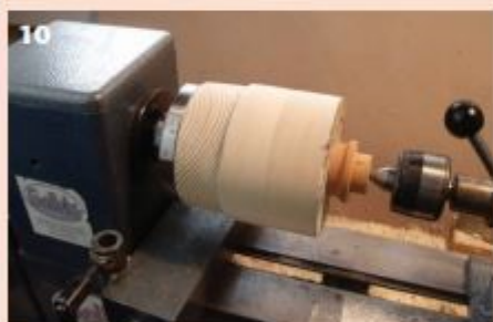
For box turning, apply hot melt glue to the base's rim and push the lid onto the rim. Turn the box as one piece.
