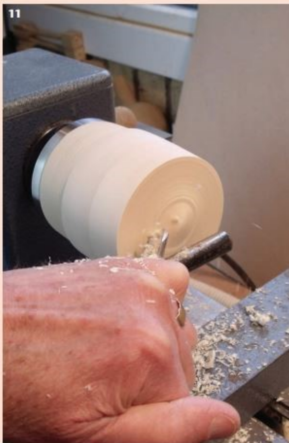
The top of the lid is accessible without the need for tailstock support.
