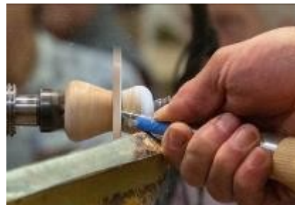
Undercutting the other side
