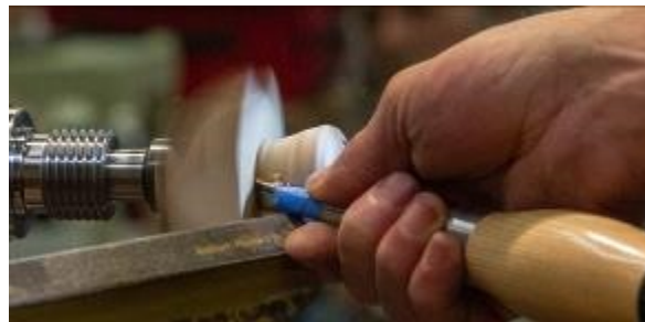
Undercutting one side
