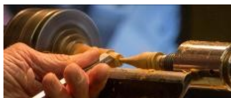
Shaping finial with bedan
