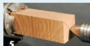
5 Mount the blank onto the lathe using a cone center in the tailstock. The butt end is mounted into a four-jaw chuck.
