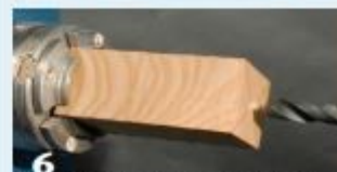
6 After turning a small depression in the end to help center the drill bit, drill a hole for the insert.
