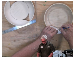
Marking out saw cuts
