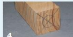
4 A block of Russian olive has the center marked and a 1" (25mm) circle drawn on one end. This will be the butt end of the handle.
