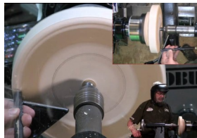
Tenon marked out, cutting curve
