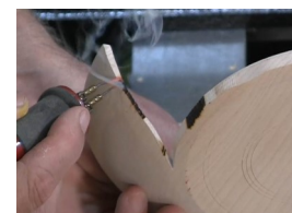
Burning treatment of edges
