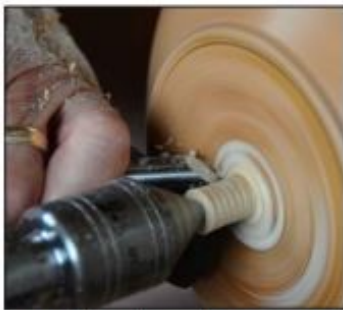
Tailstock – Tailstock live center supports bowl on the jam chuck. Leave the tailstock in place as
