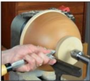
Tailstock – Tailstock live center supports bowl on the jam chuck. Leave the tailstock in place as
