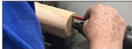
Flat pencil held flat on live center marks a 2" (50mm) circle for the chucking tenon.
