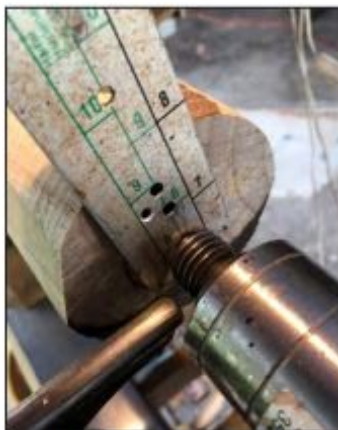
Ruler gauge has holes for each size of tenon, and a vee cut in the end that drops over the lathe center.
