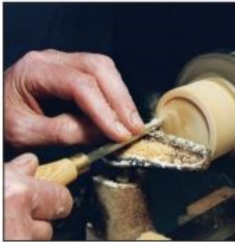
Shallow recess – Small jam chuck will be used to remount boxes and lids for cleanup.
