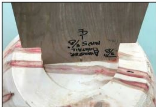
Recess gauge includes depth indicator.
