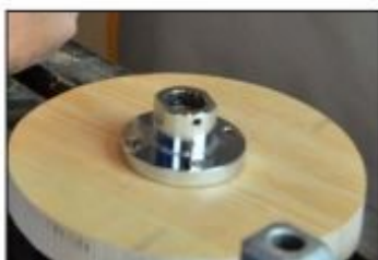
Jam chuck – To make a jam chuck, bandsaw a softwood disk and screw it onto a metal faceplate. Center, the jam chuck can be reshaped and reused many times. Right, the chuck wastes away.
