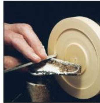
Reusable – The recess in the jam chuck is tailored to each piece in a matching set.
