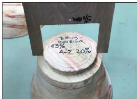
Tenon gauge nails the diameter.
