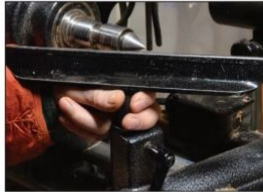
Fingers — Bring the rest up to a cone center, wrap fingers around the post, and learn how it feels. You'll quickly become able to judge center and the thickness of a tool below it.
