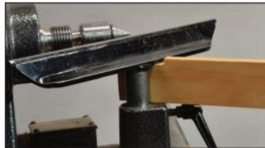
Gauge — The step gauge guarantees the rest is on center.
