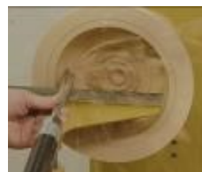
Approaching desired wall thickness
