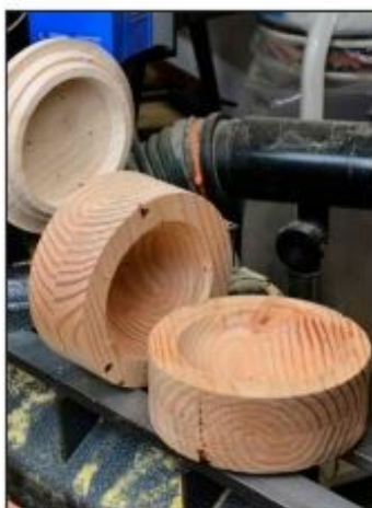
Jam chuck – To make a jam chuck, bandsaw a softwood disk and screw it onto a metal faceplate. Center, the jam chuck can be reshaped and reused many times. Right, the chuck wastes away.
