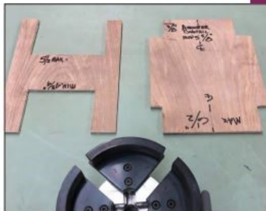
Each jaw set gets a tenon and a recess gauge.
