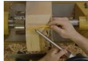
Bevel controls cut
