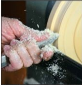
Rim shot – The bowl will fit onto a rebate turned in the rim of the jam chuck.
