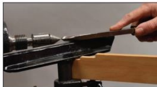
Step — The gauge step lowers the toolrest by the thickness of this scraper, positioning the edge at center height.
