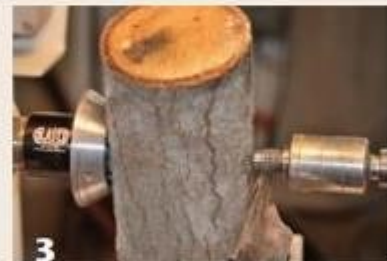
3 Mount the limb onto a screw chuck, and use a live center for support. Spin the wood a few times to be sure it is centered and does not hit the toolrest.
