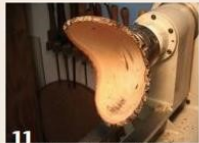
11 The inside is completed. The bowl can now be reversed in a jam chuck to finish the foot.
