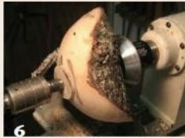
6 Complete the outside of the bowl and the tenon at the base. Remove the bark on the bottom and complete the foot.
