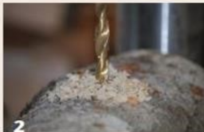
2 Drill a hole for the screw chuck.
