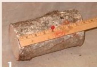
1 Cut a branch with the length one and a half to two times its diameter.
