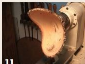
11 The inside is completed. The bowl can now be reversed in a jam chuck to finish the foot.
