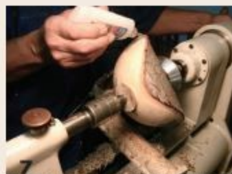
7 If necessary, apply thin CA glue to stabilize the bark. Ensure the glue has cured before starting the lathe again.
