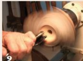
9 Take cuts from rim to base with a bowl gouge to hollow the inside.
