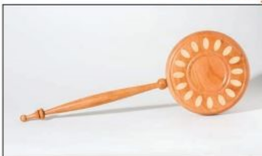
9. Inserting dowels into angled holes creates visual interest by deviating from the expected roundness of turned objects.
