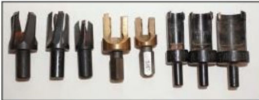
7, 8. An alternative approach is to purchase a commercially made plug cutter. With the aid of a drill press you can take an assembly line approach. Plugs can be broken free or cut free with a bandsaw.
