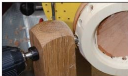
10. To create angled holes for dowels, use a shopmade jig to align the drill bit and prevent it from wandering.
