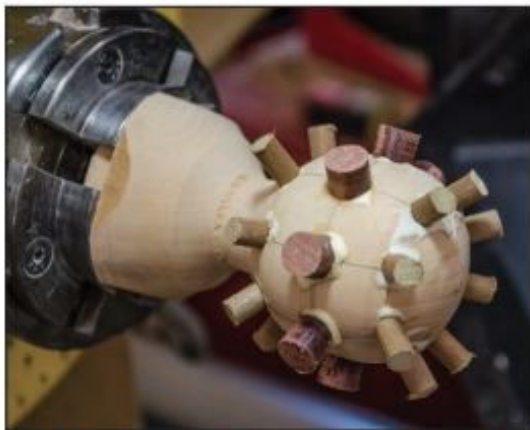
13, 14. The dowels in this ornament were laid out systematically—you can see the carefully drawn grid pattern on the blank and the resulting ordered appearance.
