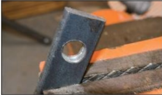
5, 6. Make a doweling jig from a small piece of bar stock. Enlarge the upper length of the hole to make starting the dowel easier--it's the bottom 10 percent (or so) of the hole that does the actual sizing. You'll need a firm clamp or vise, as force is required to drive the dowel stock through the hole.
