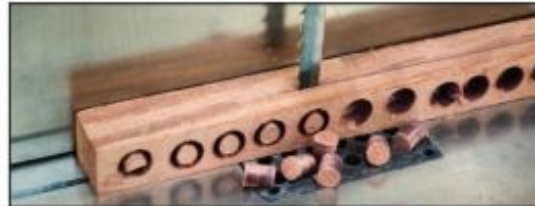
7, 8. An alternative approach is to purchase a commercially made plug cutter. With the aid of a drill press you can take an assembly line approach. Plugs can be broken free or cut free with a bandsaw.
