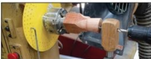
11, 12. Another approach is to drill straight holes for the dowels, then turn the object to reveal the inserted dowel. With the blank cut at an angle, the dowels themselves appear to vary in diameter.
