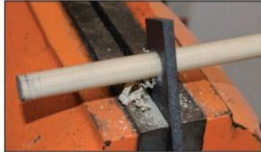
5, 6. Make a doweling jig from a small piece of bar stock. Enlarge the upper length of the hole to make starting the dowel easier--it's the bottom 10 percent (or so) of the hole that does the actual sizing. You'll need a firm clamp or vise, as force is required to drive the dowel stock through the hole.
