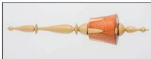
11, 12. Another approach is to drill straight holes for the dowels, then turn the object to reveal the inserted dowel. With the blank cut at an angle, the dowels themselves appear to vary in diameter.
