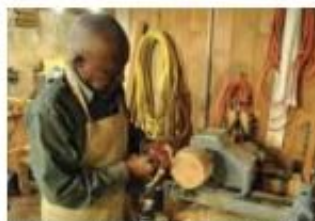
Prior to turning on the lathe, Hansel uses his fingers to gauge the position of his cutting tool in relation to the wood.
