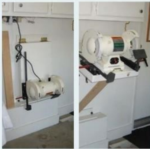
A grinder folds down out of the way when not in use, and can be easily lifted into position when needed.
