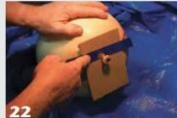
22 With the workpiece removed from the lathe, use a small hand saw to cut off the remaining nubbin of wood. A piece of cardboard protects the base.
