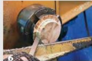
6 Mount the plug material in a chuck and form a 10-degree taper to the approximate diameter of the hole you will hollow through.
