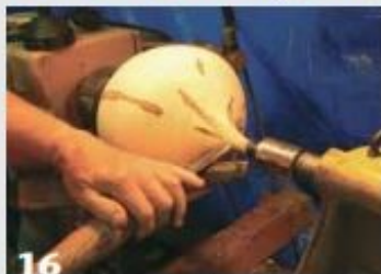
16 With the vessel now held in the chuck by the base tenon, refine the shape of the neck/spout.
