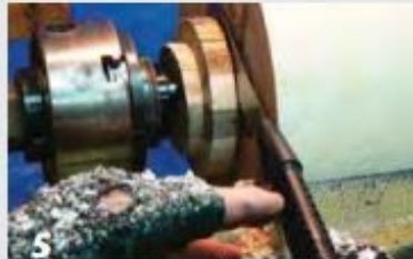
5 The author parts most of the way through next to the plug material, then finishes the cut with a hand saw with the lathe off.
