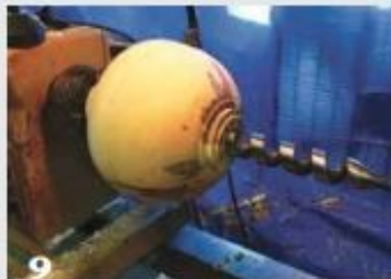
9 Reverse-mount the vessel, now holding the spout tenon in the chuck. Drill a larger hole through the bottom.
