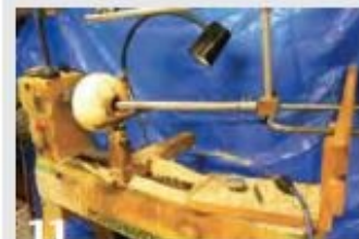
The author's hollowing rig, a captured boring bar system.
