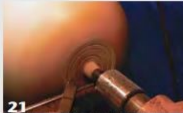
21 Carefully placed V-grooves help to hide the glue line of the plug, leaving no evidence of how the piece was hollowed.
