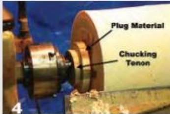
4 Use a parting tool or bedan to create a chucking tenon and a disk of material to later use as a plug. Using wood from the bottom of the workpiece will blend seamlessly with the vessel.
