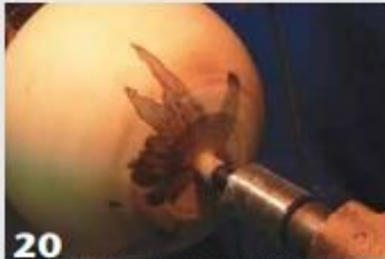
20 Turn away the plug tenon and shape the base of the vessel. Leave a small nubbin under the live center.
