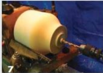
7 Mount the cylinder in a chuck, holding the tenon at the bottom. After some initial shaping, the author drills into what will become the neck, or spout.
