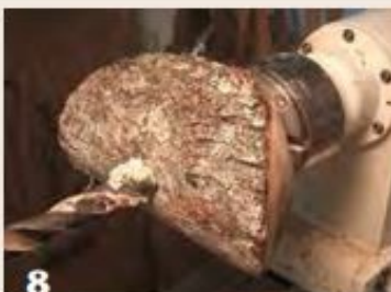
8 Grasp the tenon in a scroll chuck and drill a depth hole to begin hollowing the inside.
