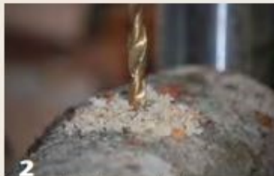
2 Drill a hole for the screw chuck.
