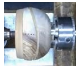
Depth holes drilled
