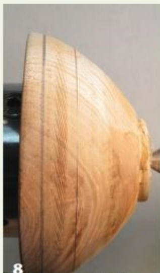
8 If the trial-start results in striations, clean off the surface and try again.
