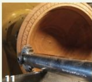
11 Use the edge of the spiral cutter to add a pattern to a bowl rim.
