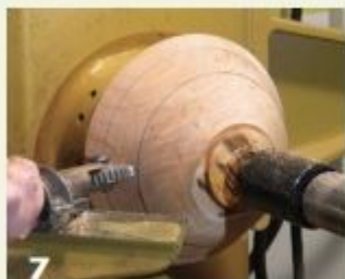
7 For spiraling on bowls, adjust the indexing saddle for a cutting angle of 15 to 20 degrees (about 1 on the index), engage the cutter, lift the tool handle, and move the tool along the toolrest.
