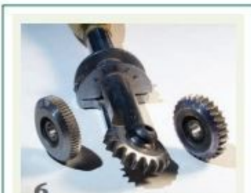
6 Spiraling cutters look like gears. The adjustable indexing rest makes it easy to control the cutting angle and to accurately deepen cuts.
