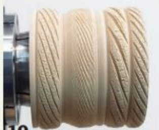
10 These rope patterns on a spindle illustrate what you can do with different size spiraling wheels over a bead.
