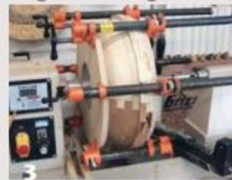
The author constructs the vessel one segmented ring at a time, using the lathe as a holding device during glue-up and turning the form in stages.
