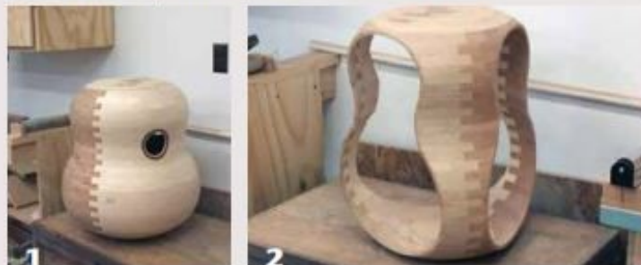
The author's vision: Turn a guitar-shaped vessel, then slice off sections of it to create contoured soundboards.
