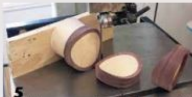
Soundhole accents are inserted, then turned flush before construction of the vessel continues.
