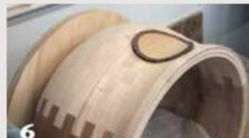
Soundhole accents are inserted, then turned flush before construction of the vessel continues.
