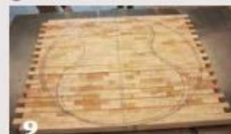
A segmented board is turned to thickness, then cut to shape and used as the guitar back.
