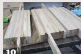
The author glues up several boards from which he cuts out the guitar sides.
