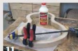
To cut out the inside of the form at the bandsaw, a kerf through the side is necessary to provide blade access. After cutting the inside shape, the kerf was closed back up with glue.
