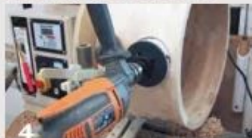
The segmented form, once built past the soundhole location, is bored with a hole saw.
