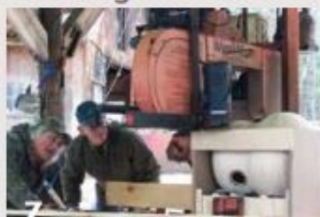
The author (right) employs the use of a local sawmill to slab off the three soundboards. Note the specially made jig for holding the vessel safely during cutting.
