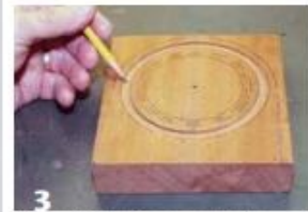
3 Shape the inlay ring to match the dimensions of the recess it will fill.
