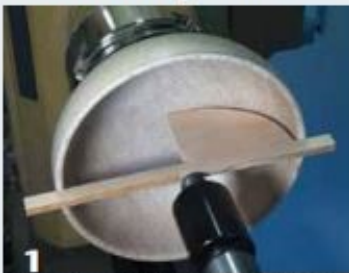
1 Create a paper pattern on a plywood support to capture the inside and outside profiles of a bowl.
