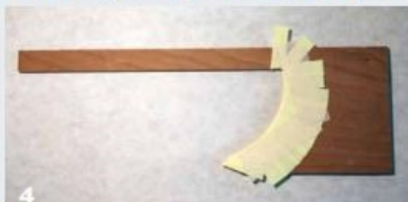
4 Reinforce the paper pattern with tape.
