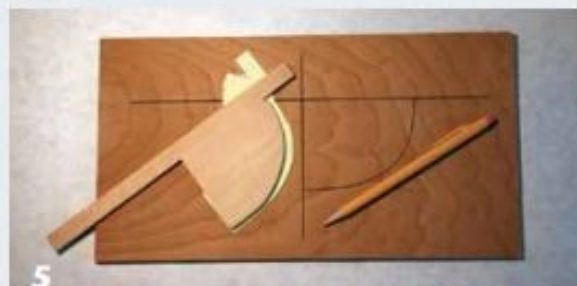
5 Trace the pattern onto your final template material, then cut it out and start duplicating at the lathe.
