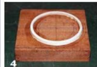
4 Glue the inlay ring into the routed recess.
