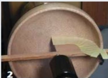
1 Create a paper pattern on a plywood support to capture the inside and outside profiles of a bowl.
