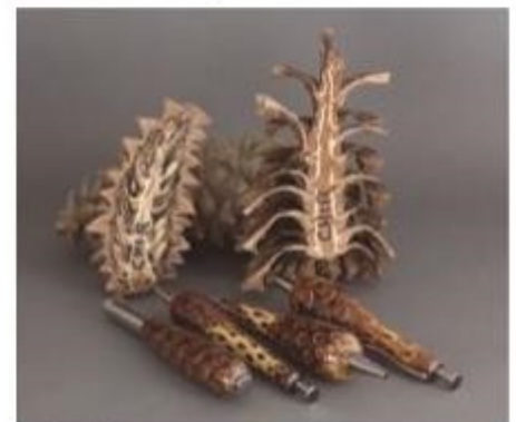
Each of these pens was made from an open Chir cone similar to the cut cone to the right. The smaller closed cone at the left shows the seed area that presents turning challenges.
