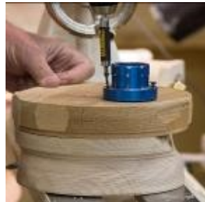
Faceplate From Center to Offset Position #1
