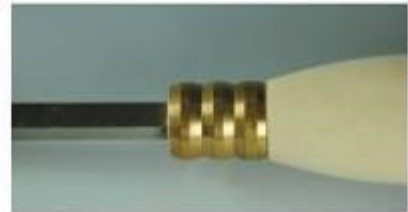
This ferrule is made from three brass natural-gas fittings.
