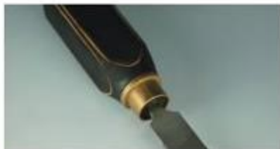
This ferrule is a bushing from an electric motor shaft. They come in a variety of sizes.
