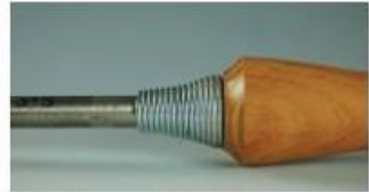
This ferrule is a spring that was removed from the screen door of my home.
