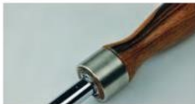
This stainless steel ferrule came from pipe that I salvaged from a boat. Stainless steel is hard to cut but it is strong and looks good with any wood.
