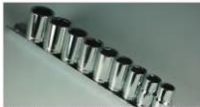
I often buy a set of sockets when re-handling a set of bench chisels. I use the smaller socket for the smaller chisels and the larger socket for the larger chisels.
