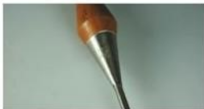
This ferrule started out as a tip used for frosting cakes.
