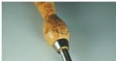
A spacer-lug from a truck tire becomes a sturdy ferrule.
