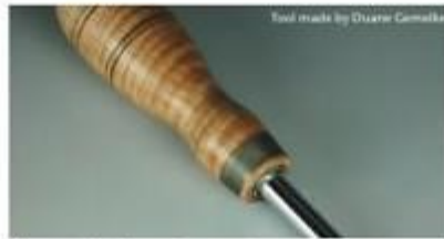
Wrapped piano wire creates a unique appearance that goes well with highly figured wood.
