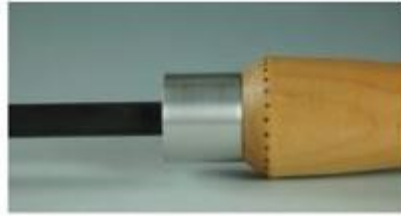
Aluminum is easy to cut and readily available—it is a good starter ferrule.
