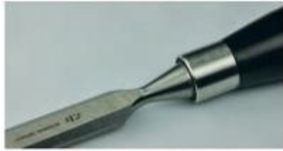
Stainless steel is a favorite ferrule on a chisel because it can withstand pounding and levering.
