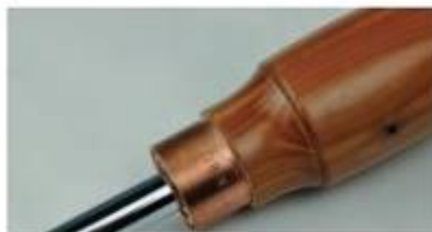
This copper ferrule has developed a warm patina over time. I often select a ferrule that will complement the wood.
