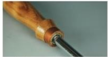
I used a pipe cutter to add a shallow cut to the end of a copper ferrule, a detail that I often use.
