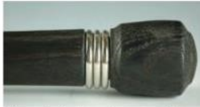
A decorative ferrule transforms a roughing gouge. I joined two pieces of ebonized red oak with a tongue-and-groove joint and sandwiched the ferrule in between.
