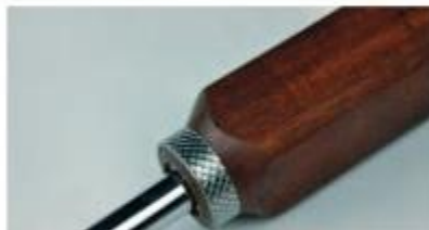
I cut this ferrule from a textured bathroom towel bar.
