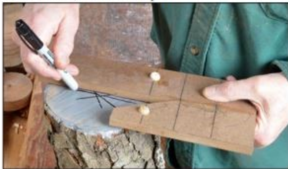
Photo 2. Bill of materials: MDF 1/2" x 2-1/2" x 11" and 2-1/2" x 6" cut 30°, two 1/2" dowels spaced 2-3/4" apart, #0 joinery biscuit.
