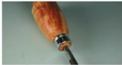
This ferrule started out as an aerator on a kitchen sink faucet. The ultimate repurpose.
