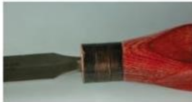
Three separate pieces of ebonized copper pipe butted together make a utilitarian ferrule. With use, the black wears off and the ferrule develops a fine patina with the copper showing through.
