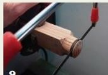
9 Part off the disk with a thin parting tool or fine-toothed saw with the lathe off. Hand sand the nubbin.
