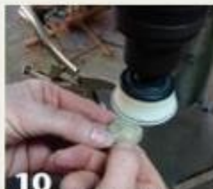
10 As a sanding alternative, chuck a sanding disk in the drill press and sand the rough areas on the back side.
