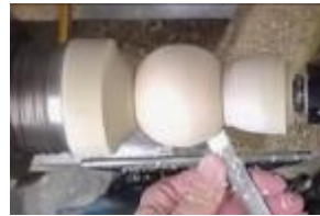
Smoothing with skew chisel
