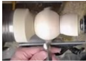
Turning off tenons
