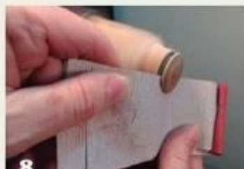
8 Sand the right side, the upper edge, and as much of the left side as possible.
