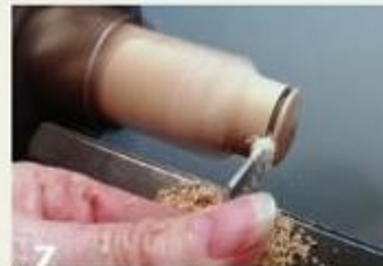
7 Use a thin parting tool, aimed slightly toward the headstock, but do not completely part off the disk.
