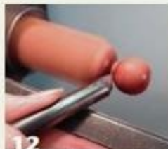
12 Use a spindle gouge or skew to turn the bead. Sand and apply friction polish or wax before parting it completely off.
