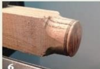
6 To turn smaller disks in endgrain orientation, mount a blank with the grain running parallel to the ways of the lathe into a chuck with small jaws. Round part of the blank into a cylinder and create a convex surface on the end.
