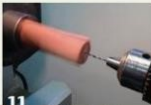
11 To turn endgrain beads, start by drilling a center hole.
