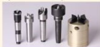
From left: Stebcenter (spindles, dry wood); shallow-fluted, four-prong center (spindles, bowls, dry wood); deep-fluted, four-prong spur drive (spindles, bowls, vessels, green or dry wood); circle drive (spindles, bowls, dry wood); 2", four-prong spur drive w/ removable blades and point (large bowls, vessels, green or dry wood).
