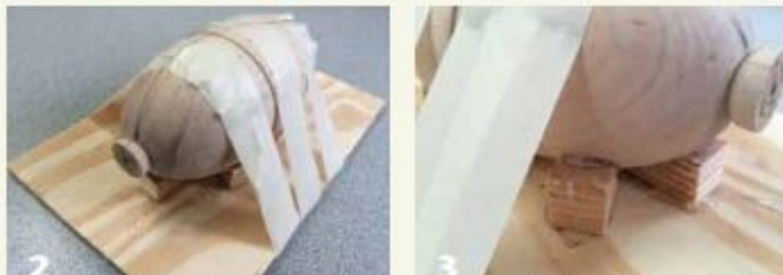
2 Workpiece is glued and taped to the wedges and carrier, ready to be cut apart on the bandsaw. Note the intended cut line for this pod form (along the sidegrain). The jig can also be used to cut across the grain to remove a tenon.
