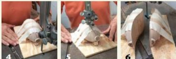
The author's pod cut in half on a curved line. The tenons at each end can be cut off after the pod is split.
