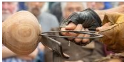
Checking wall thickness
