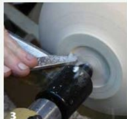
This picture shows the tool can be used even with a live center in the way.
