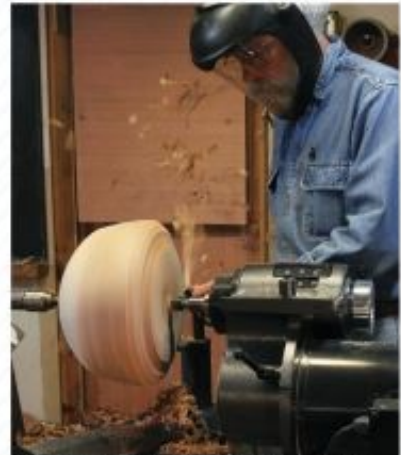
You can rough out a moderately large form (either green or dry wood) with just a 1" (25mm) deep-fluted, four-prong spur drive without fear of losing the piece.
