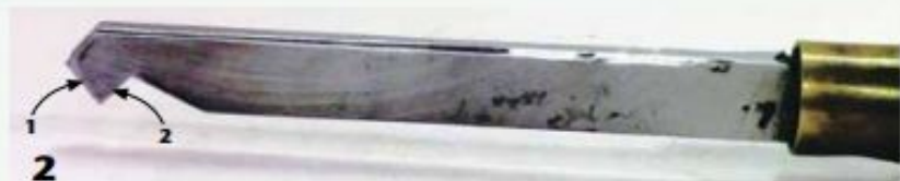
The author's shopmade dovetail recess tool, made from an old skew 1/2" (13mm) wide and a bit less than 1/4" (6mm) thick. Edge 1 forms the bottom of the recess, and edge 2 forms the angled wall. The angle between these two edges should match the angle on the outside of your dovetail jaws (in my case, about 80°). Since edges 1 and 2 are being used as scrapers, their bevels should be ground at a 70° to 80° angle.
