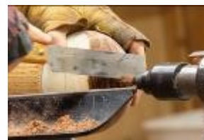
Removing excess tenon
