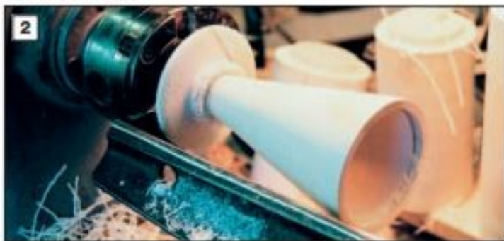
2 Mount the body in a scroll chuck, using the tenon. Shape the body first, then hollow the interior with a 1/2" spindle gouge. Hollow the interior to reduce weight—just in case someone wants to use the angel as an ornament. To mount the body with a scroll chuck in the next step, turn a spigot on the inside of the body.
