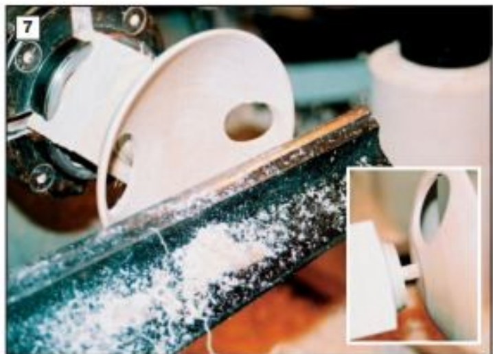
7 Use a 3/8" bowl gouge to turn the interior of the bowl-shaped wings. When finished, turn a 1/4" tenon (inset) on the back side of the wings. The wings attach to the body with the tenon.
