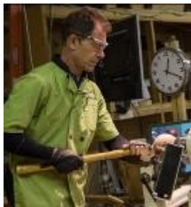
Proper stance for hollowing
