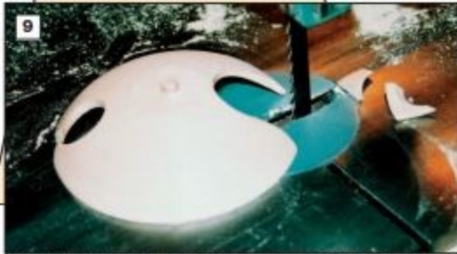
Using the pattern above as reference, cut the final wing shape with a bandsaw, scrollsaw or coping saw.
