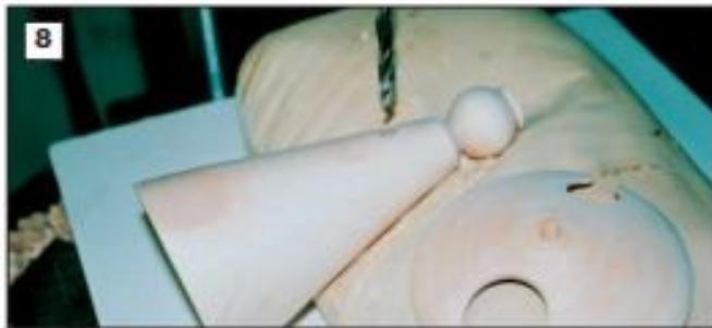
Prop and support the angel on a sandbag, then drill a 1/4" hole in the back of the body to fit the wing tenon. Use your hand to prevent the angel from rolling during the drilling procedure.
