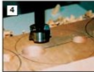
4 Before cutting circles for angel wings, mark a centerline on a 5/4" \times 4" wide maple or ash stock. Draw a 3 1/2" circle and mark center for the 3/4" and 1 1/8" holes. Then bore the holes with a Forstner bit as shown.
