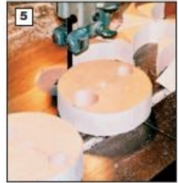
5 After boring the holes, bandsaw the 3 1/2" -diameter wing discs.
