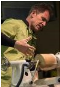
Blank mounted between centers
