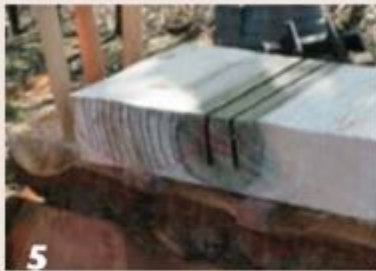
5 The center section of the log, next to the pith area, yields quartersawn blanks. Depending on the size of the blank and your bandsaw, it may be possible to take the log section straight to the bandsaw for sectioning.
