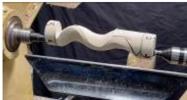
Arc cuts with parallel axis
