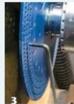
The author's shopmade locking pin, affixed in a base on the lathe bed, provides a positive hold for accurate indexing.
