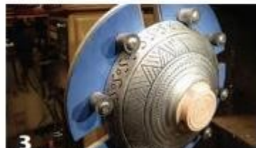
The author's Nick Agar-style bowl, reverse-mounted for finishing its base. In some cases, this method may be preferable to using a vacuum chuck, which could damage the paint on the inside.
