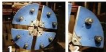
Craft foam adhered to jumbo jaws protects bowl rims.
