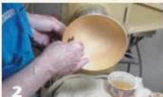
2 Sanding with water as a lubricant works especially well on green-wood turnings like this once-turned, very thin bowl.
