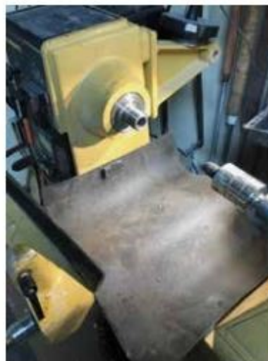
The author's Nick Agar-style bowl, reverse-mounted for finishing its base. In some cases, this method may be preferable to using a vacuum chuck, which could damage the paint on the inside.
