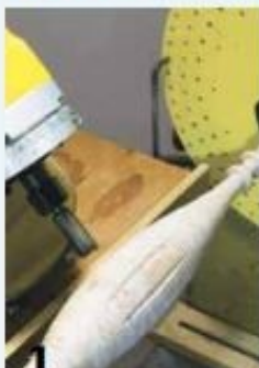
A router on an auxiliary table can be used to make repeatable cuts in a workpiece. The index wheel and locking pin ensure consistent spacing.
