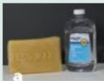
Melted beeswax and mineral oil make a fine sanding paste that will help keep sanding dust down and create a very smooth surface.
