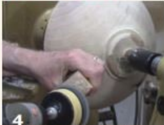
4 Clean sanding disks on a power sander by running them against a sanding belt cleaning stick.
