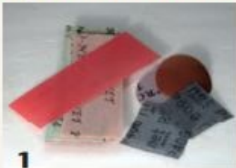
1 Open-mesh abrasives like Abranet or Wonder Weave work great for wet-sanding. They don't clog as quickly as cloth- or paper-backed abrasives, and they are easy to clean out and reuse.
